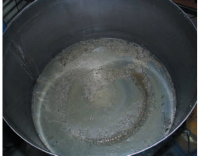
Fig. 8 View from above into the sediment chamber showing the wake devoid of sediment that is observed after a ploughing experiment. The direction of ploughing is counterclockwise.
