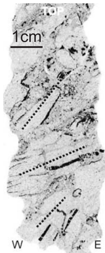
Fig. 4 Sample LD1, thin section. Linear features marked by coal alignment are indicated with dotted lines. East and west are indicated at the bottom of the picture.
