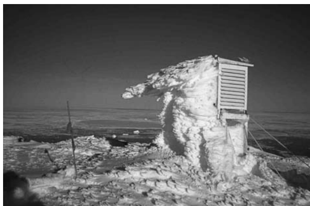
Fig. 4.34 A weather screen on Mt. Coburg, Arctic Canada ( 76^{\circ} N, 79.3^{\circ} W) heavily coated with rime ice. Open water in the North Water, Baffin Bay (visible in background) provides a moisture source in spring. The air temperature was -15^{\circ} C (K. Steffen).
