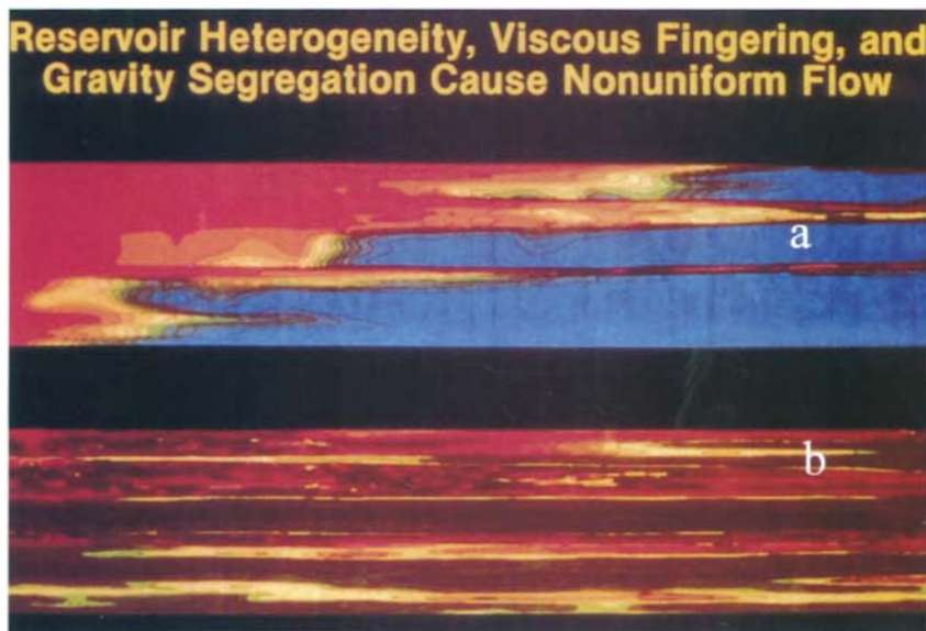
FIG. 8. Calculated flow behavior for injection of CO 2 into a heterogeneous oil reservoir resulting in viscous fingering under the combined effects of gravity and heterogeneity. The lower panel (b) shows the spatial distribution of permeability in the two-dimensional cross-section. The upper panel (a) shows the portion of the reservoir invaded by CO 2 . The low-viscosity CO 2 invades the higher permeability zones preferentially, and gravity forces cause the lower-density CO 2 to invade the upper zone as well. Similar behavior will occur in aquifers (K. K. Pande, personal communication).
