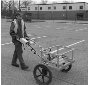
Fig.1. Operator equipped with EM61-MK2
