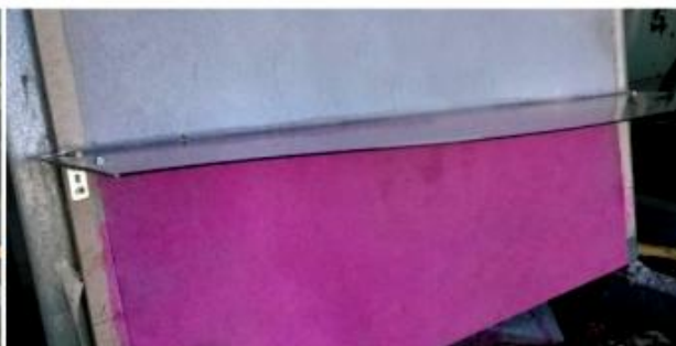
Time zero: Photocatalytic panel exposed outdoors. The purple section is treated with a pollutant (Rhodamine B). A small plexiglass roof protects the treatment from being washed away by the rain.
