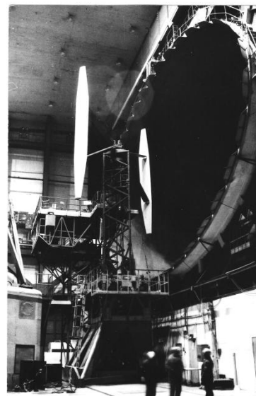
Fig. 13 – Two-blade orthogonal unit on tests in TsAGI
