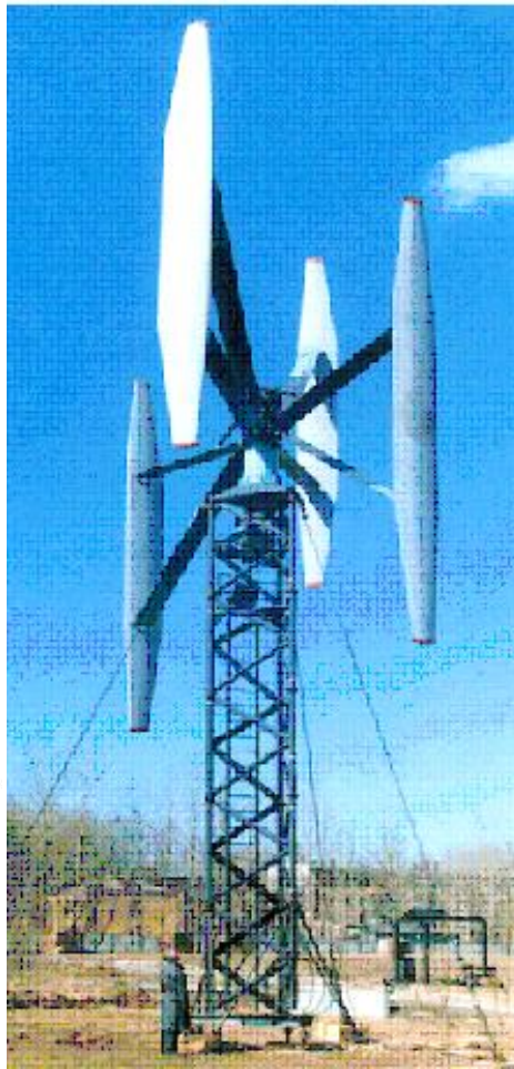
Fig. 36 – Network wind turbine with a gear-motor 50 kW and two tiers with two blades each
