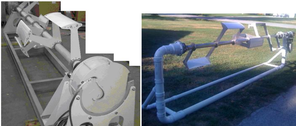
Fig. 2 – Orthogonal hydro turbines with a horizontal axis
