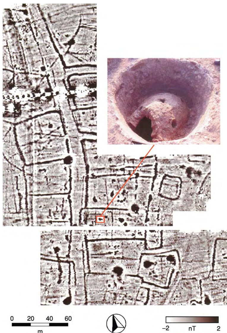
Figure 2 Sedgefield, County Durham. Fluxgate gradiometer data. 1 \times 0.5 m. Romano British settlement straddling a road. Excavation by Time Team revealed a complex of workshops and a small kiln as highlighted in the inset photograph. (Reproduced from Gaffney C and Gater J (2003) Revealing the Buried Past: Geophysics for Archaeologists , Tempus Publishing Ltd (Plate 19).)
