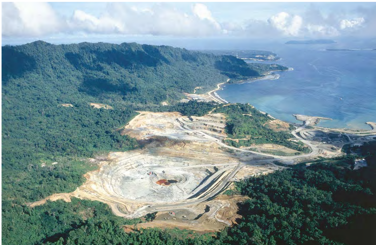
Figure 9 The open pit gold mine at Lihir Island, Papua New Guinea, under development in 1998, twenty months after inception of mining operations. The two pits, then about 40 m deep, and centred on ore bodies 1.5 km apart, will merge into a pit about 2 km across, with a planned depth of 300 m. The background and foreground hills are the walls of the volcanic caldera in which the epithermal gold pyrite mineralization occurs. Photograph by courtesy of Rio Tinto PLC. Reproduced with permission from Evans AM (1995) Introduction to Mineral Exploration . Oxford: Blackwell p. 34.
