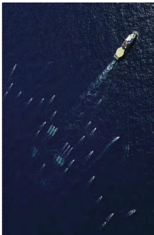
Figure 7 Aerial view of an offshore seismic survey, showing the array of hydrophones being towed behind the ship. Reproduced with permission of Millenium Atlas Company Limited.
