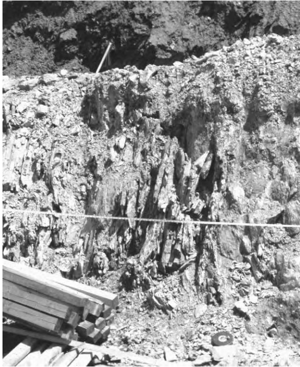
Figure 2 An example of a zone of 'bad ground' discovered and delimited in an engineering geological site characterization exploration. This zone represents poor engineering properties of foundation materials in terms of their ability to support structural loads that would be imposed by engineered works. Shown is a shear zone of ancient tectonic origin, as it perpendicularly enters the foundation excavation for the Lahey Medical Clinic, urban Boston, Massachusetts. Such features are important when they are planar to and cross one or more dimension of the foundation excavation, because they have the potential to induce instability of the surrounding ground and existing buildings. Timbers are 200 mm 2 in section; survey tape in midview. Photograph by the author.
