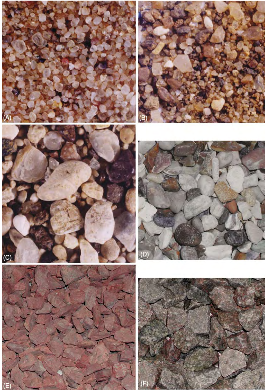
Figure 1 Aggregate grades. (A) Fine sand suitable for mortars or render (width of image: 10 mm). (B) Coarse sharp sand or 'concreting' sand (width of image: 10 mm). (C) Coarse natural sand (width of image: 10 mm). (D) Flint gravel 5–10 mm (width of image: 100 mm). (E) Crushed granite 5–10 mm (width of image: 100 mm). (F) Crushed granite 10–20 mm (width of image: 100 mm).
