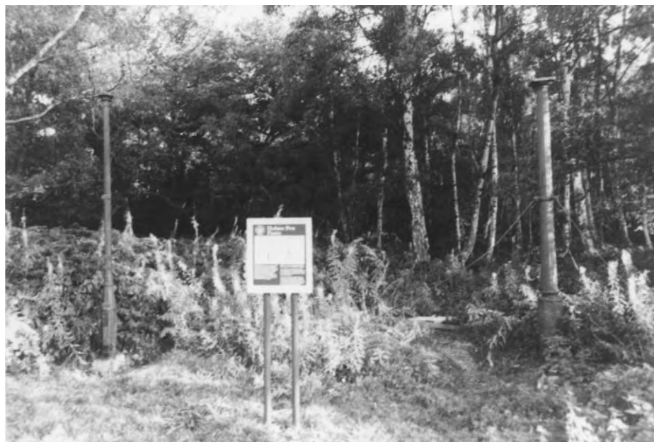
Figure 9 Holme Post, a cast iron pillar erected in 1851 on the south west edge of Whittlesey Mere, near Peterborough, England, to indicate the amount of peat shrinkage and associated subsidence caused by drainage. The post was driven through 7 m of peat into clay until its top was flush with the ground. Within 10 years ground level had fallen 1.5 m through shrinkage. A second post was erected in 1957 with its top at the same level as that of the original post (right hand side). Between 1851 and 1971 the ground subsided by some 4 m.
