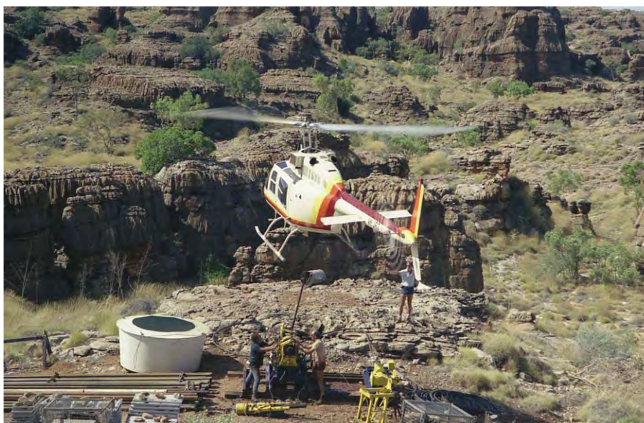
Figure 6 A helicopter being used to move a diamond drilling rig in the Kimberley region of Western Australia. The helicopter allows the drill to be positioned with minimal disturbance and environmental damage.
