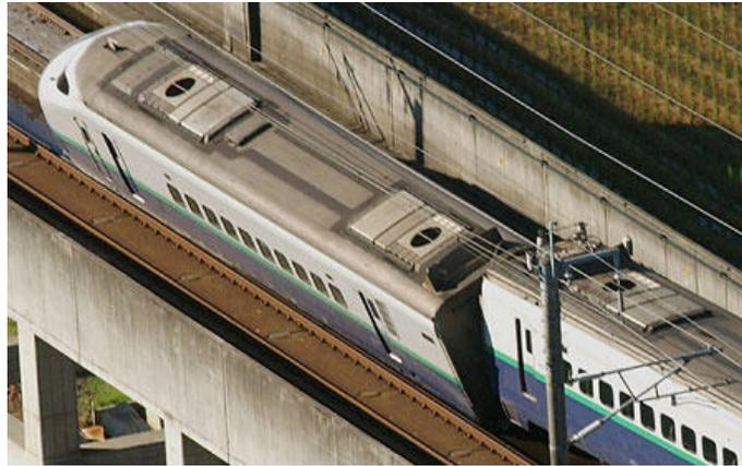
Figure 1. Derailment of a Shinkansen high-speed train during the Niigata Earthquake [4]
