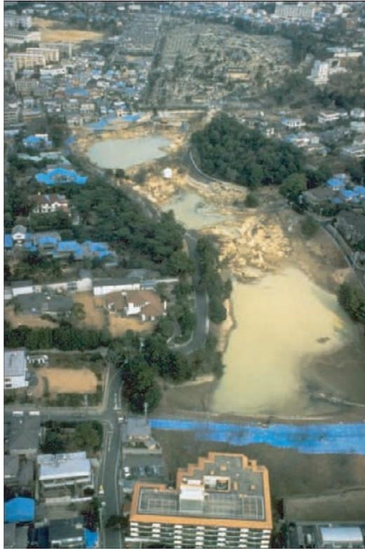
Figure 20. Niteko earth dams complex, after the Kobe earthquake (1995). (Courtesy of the National Information Service for Earthquake Engineering, EERC, University of California, Berkeley).
