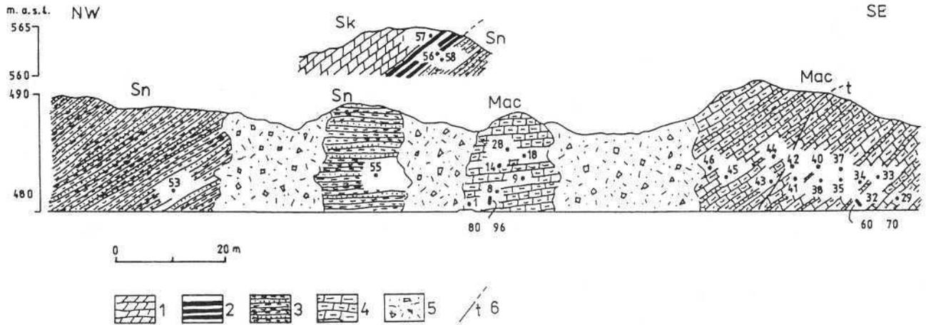
Fig. 19. Geological cross-section of the Pieniny Succession at the Macelowa Góra Mt above the Dunajec river (Bąk, 1995b). Skalski Marl Member (Sk), 1 - variegated marl, 2 - grey-green and black marly shales, 3 - Snežnica Siltstone Member (Sn), 4 - Macelowa Marl Member (Mac), 5 - weathered material, t - larger faults.
