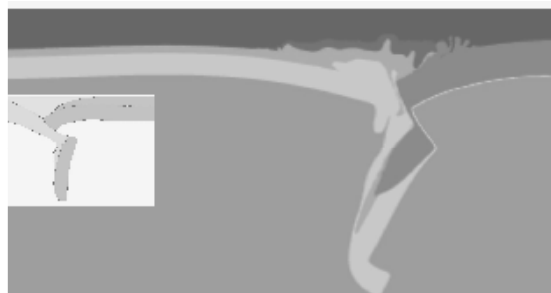
Fig. 2. Break of the accreted terrain edge during subduction restarting (to the right island, to the left oceanic plate), numerical modeling from (Simakin, 2014). Results of the analogous modeling from (Boutelier and Chemenda, 2011) are in the inset.
