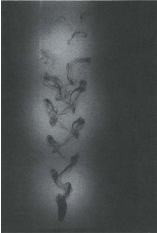
FIG. 3.15. Experimental photograph of a falling short cylinder at Re = 70 . (Photo courtesy of Dr. K. O. L. F. Jayaweera.)
