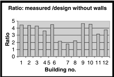
Fig. 8.9.b. Ratio of frequencies for the cases with and without infilling walls
