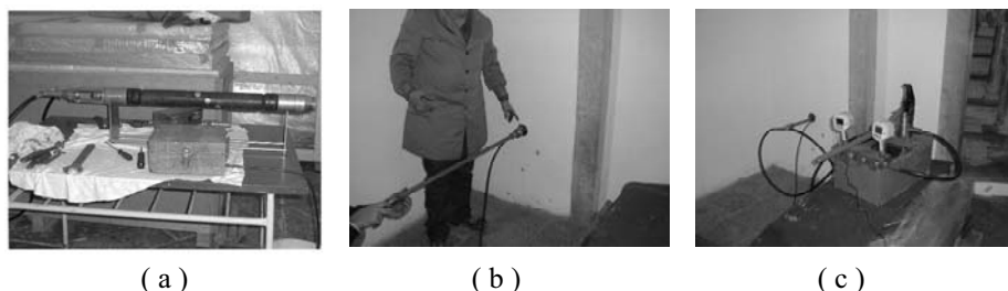
Fig. 19.15. Dilatometric test: (a) the equipment; (b) setting the equipment; (c) performing the test
