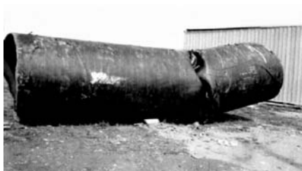
Fig. 14.4. The Sea of Marmara earthquake. Effects of surface faulting on a 2-meter diameter water main. Courtesy of Prof. Polat Gulkan
