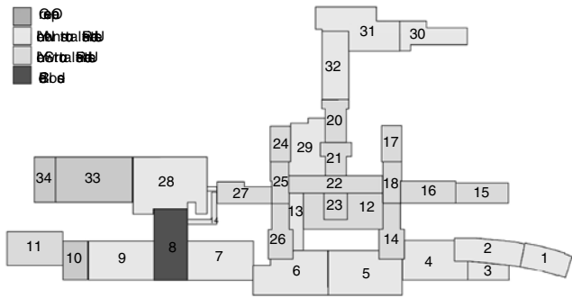
Fig. 16.17. Hospital plan showing expected performance for each building for a MCS Intensity VIII (MCS) scenario. (ATC-51-1, 2002)
