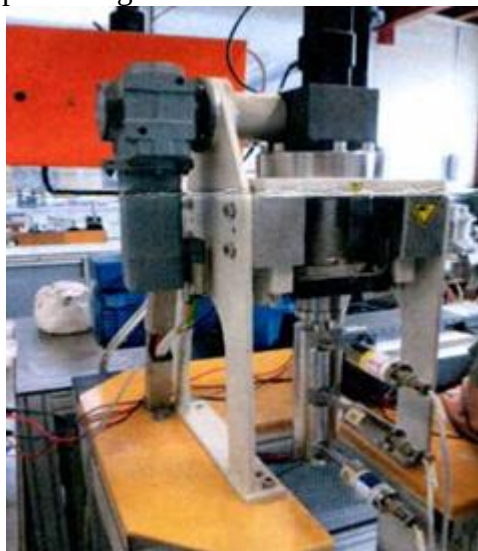
Fig. 1 Capillar Check with measurement barrel and connected pressure transducer
