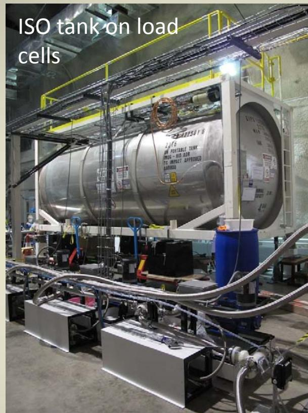
Detector target filled from GdLS in ISO tank.
