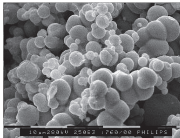
Figure 2. SEM image of tantalum carbide microspheres.
