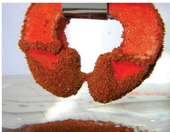
Figure 1. Magnetic nanocomposite MMN200 based on biporous commercial sorbent.
