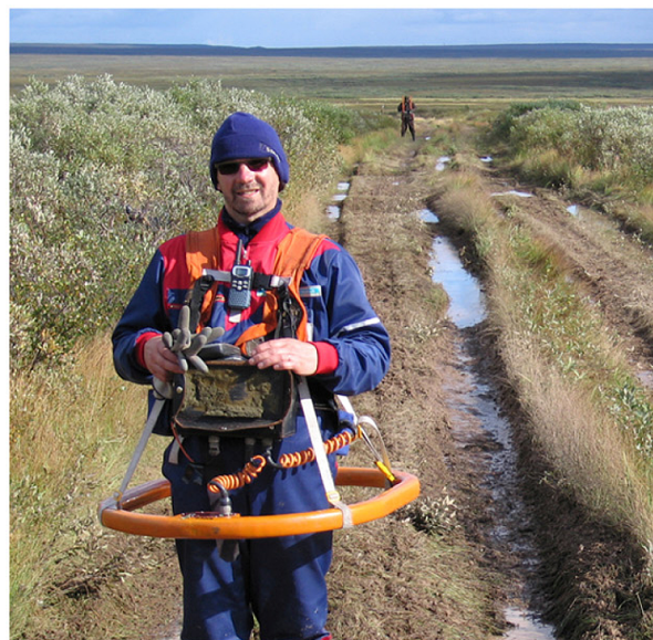
Electromagnetic survey at Mireko's Lek Vorkuta research site in 2007. Electrical sections show mostly permafrost, but also taliks (unfrozen ground)
