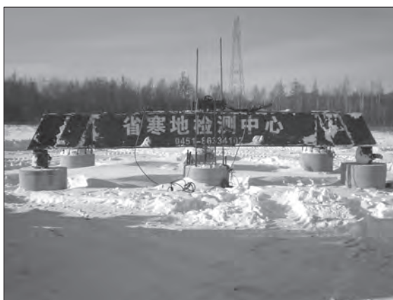
Fig. 3. Vertical steady pulling of separate pile.
