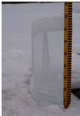
Fig. 6. Estimated extinction coefficient for Lake Pääjärvi ice in 18 March – 2 April 2003. The photograph on the right shows the ice sample in normal light, the top snow-layer and lower clear congelation ice are well seen
