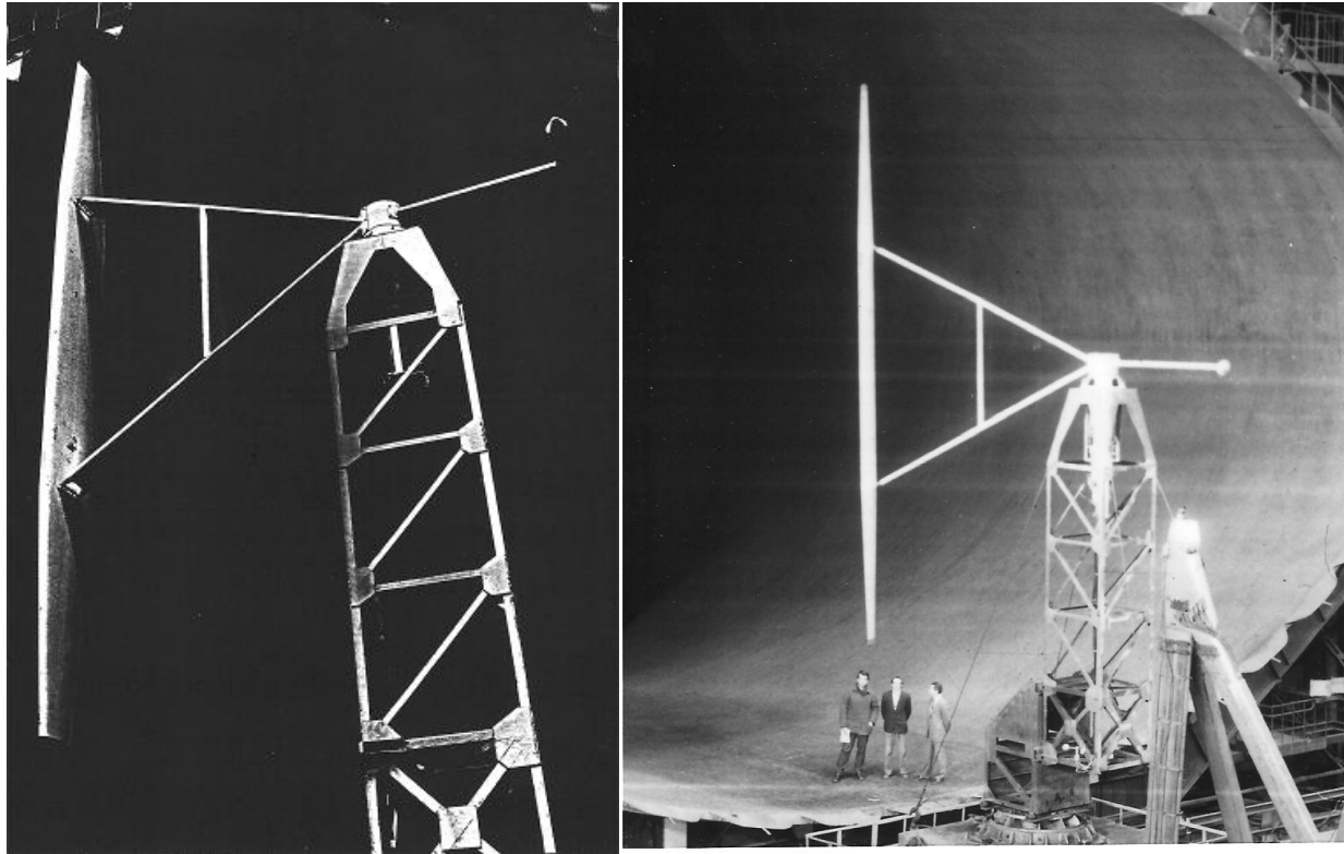
Fig. 31 – Orthogonal single-blade wind turbines to the test in the largest pipe TsAGI: the radius of the track of the blade – 3.54 m; blade area – 6.4 m 2 ; the average chord – 0.74 m; length of the blade – 8.6 m; the profile NASA0021
