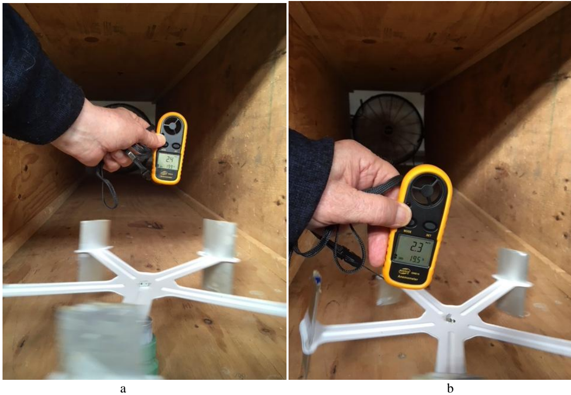
Fig. 44 – The wind speed outside the multi-blade turbine (a – U = 2.4 m/s) is almost the same as in front of the rear line of the blades (b – U = 2.3 m/s) in the turbine with 5 blades whose height (from the support to the end) is 10 times smaller than the diameter of the turbine
