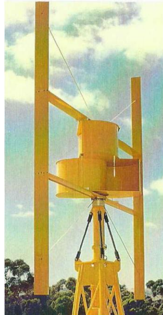
Fig. 38 – Orthogonal wind turbine with acceleration turbine Savonius on the axis
