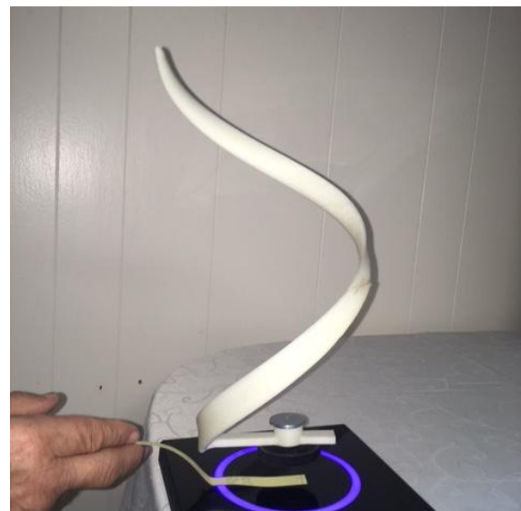
Fig. 42 – Spiral turbine model on magnetic suspension
