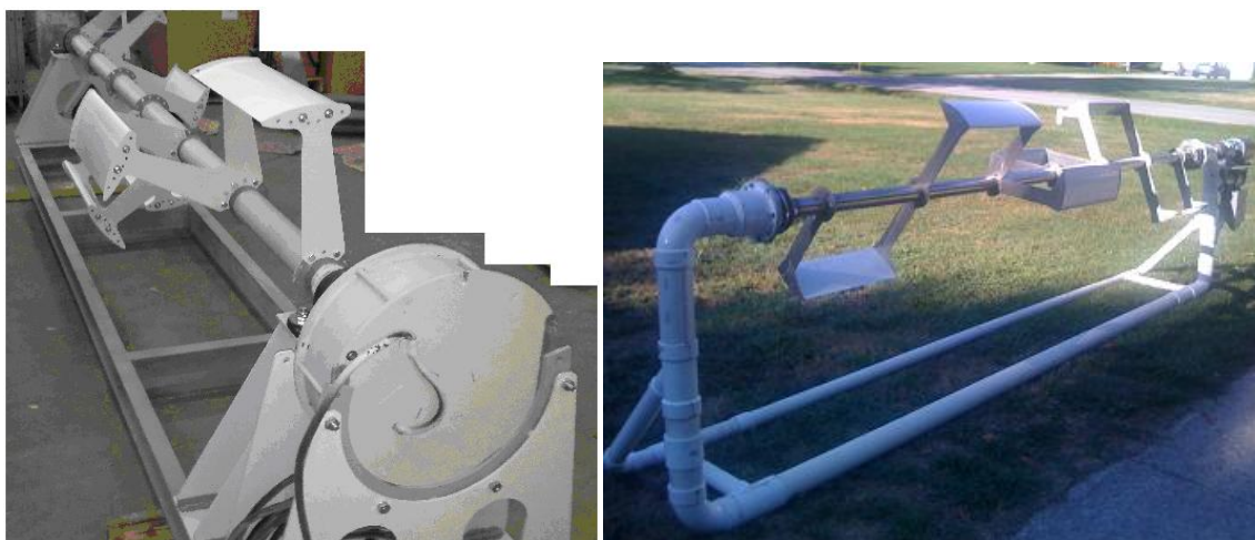
Fig. 2 – Orthogonal hydro turbines with a horizontal axis
