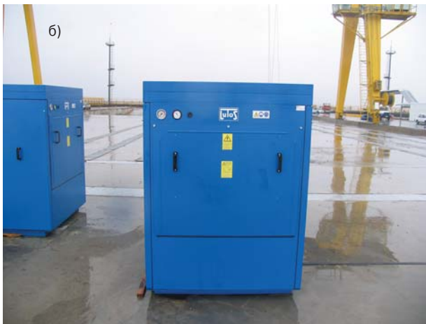
Fig. 4. General view and system of aeration of the complex of biothermal treatment at the Mikhailovsky-Kokhanskoye deposit of Samaraneftgaz OJSC: a – a general view of the complex with air channels; b – blower for stack aeration; c – aeration channels
